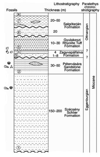
FIGURE 3. Generalized Miocene stratigraphy of the Ipolytarnóc area (after Bartko, 1985; Pálfy, 2007). Lithology: 1, silty and clayey sandstone; 2, glauconitic sandstone with conglomerate lenses; 3, pebble conglomerate; 4, trackbearing sandstone; 5, rhyolitic ignimbrite; 6, redesposited tuff and sandstone; 7, variegated clay; 8, sand.
